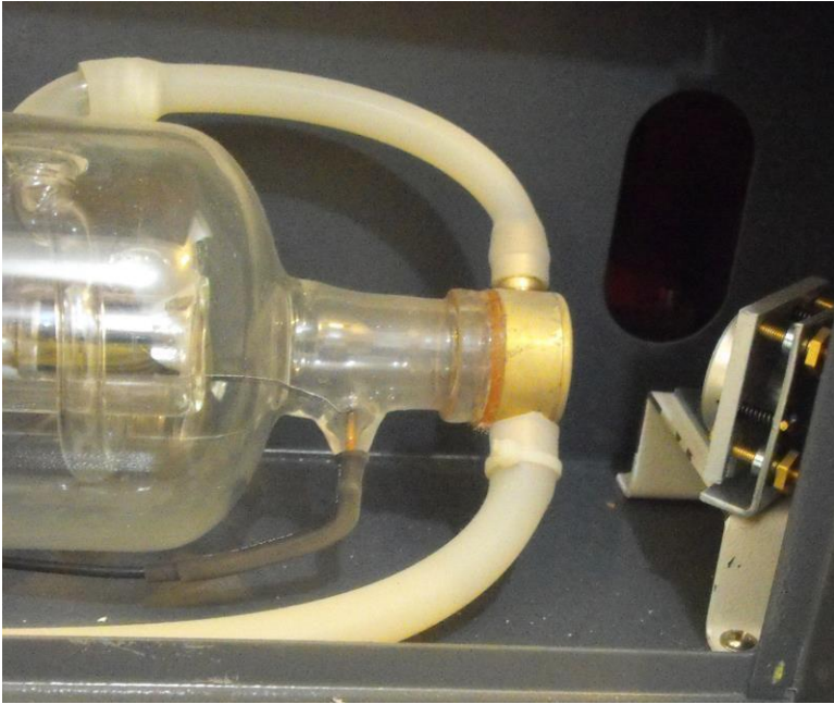
Output of Laser showing black cathode wire running along the tube, back to the power supply.
