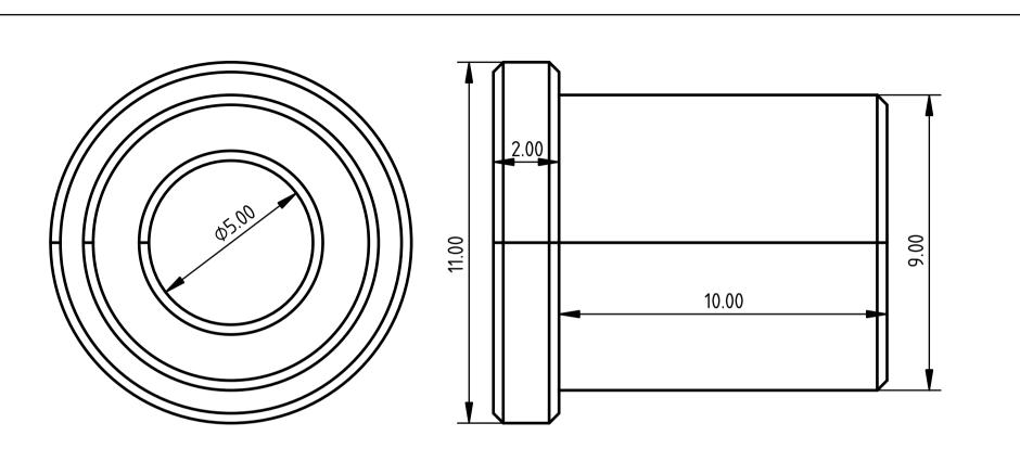
Chamfer all edges (including bore), approx. 45° x 0.3, by eye
