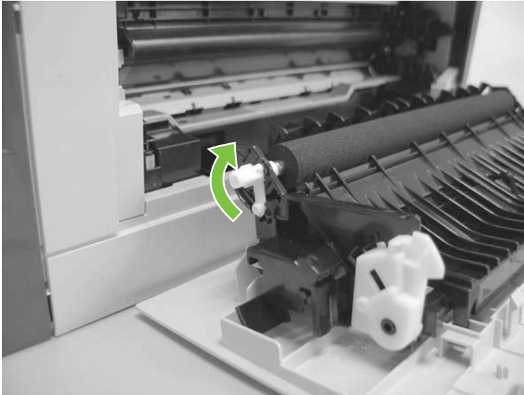
Figure 6-7 Remove the transfer roller (1 of 3)
