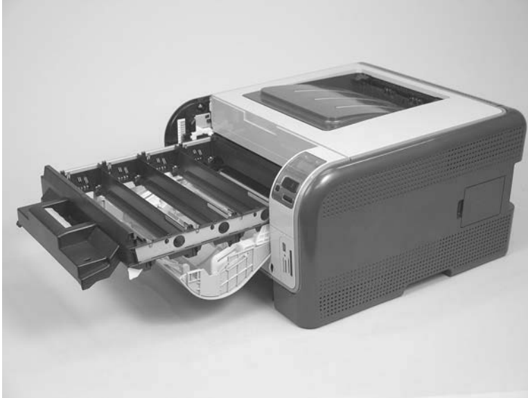
Figure 6-48 Remove the ITB (1 of 9)
