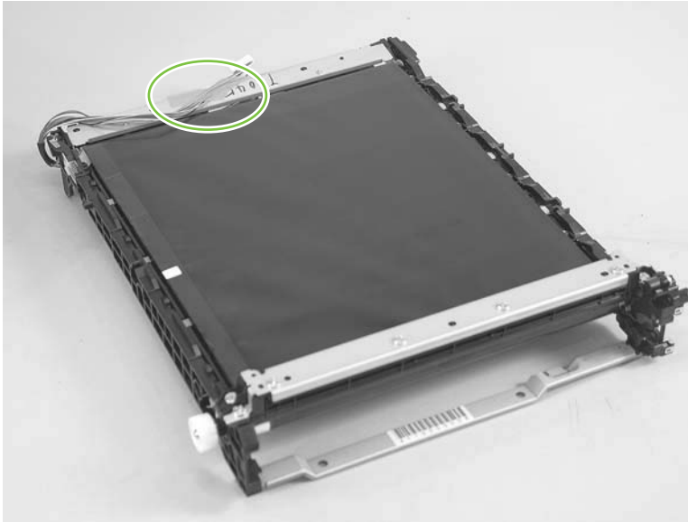
Figure 6-58 Reinstall the ITB (2 of 2)
