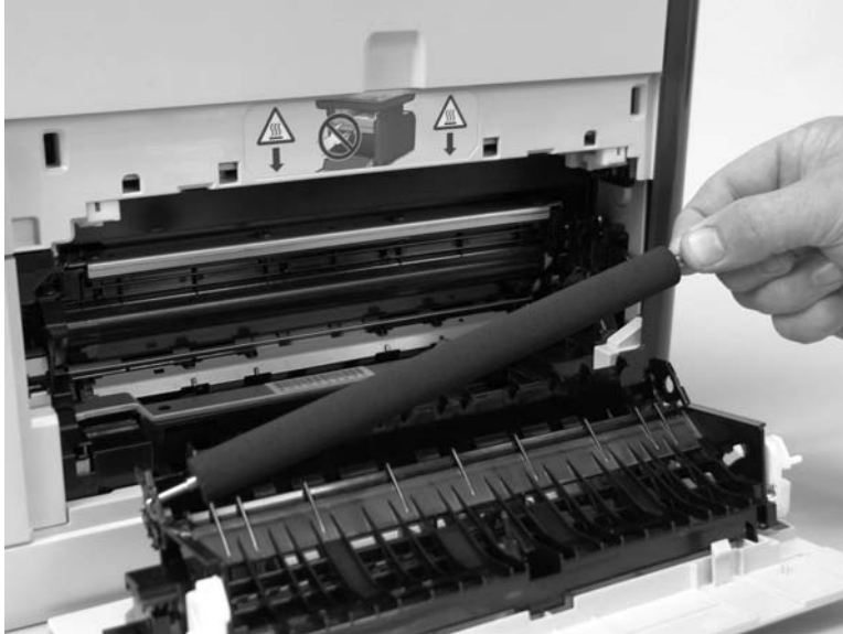
Figure 6-9 Remove the transfer roller (3 of 3)
