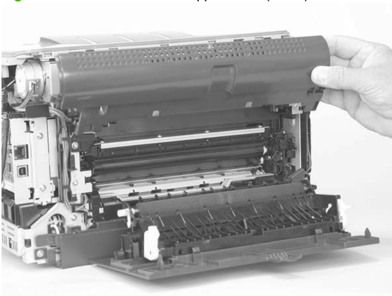
Figure 6-35 Remove the rear-upper cover (2 of 2)
