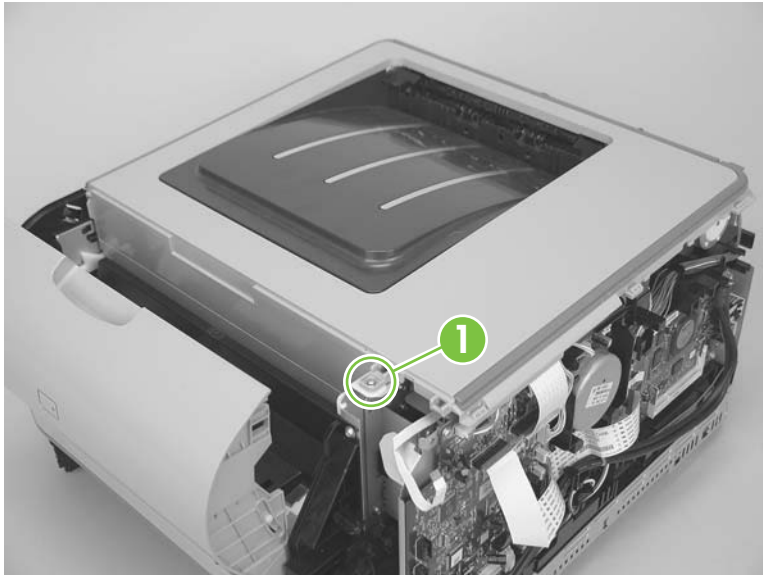
Figure 6-40 Remove the top cover (1 of 4)
