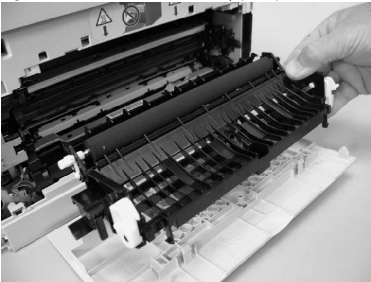
Figure 6-11 Remove the feed assembly (2 of 2)
