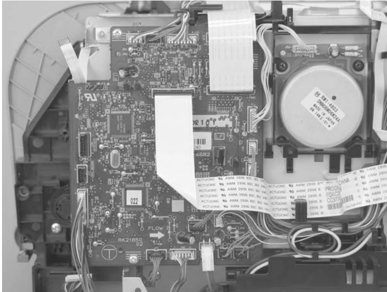
Figure 6-60 Remove the DC controller PCA (2 of 3)
